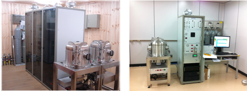
Fig. 5.2 Fixed radioactive Xe monitoring system(SAUNA II-IMS) and analyzer for mobile sampler(SAUNA II-Lab)
