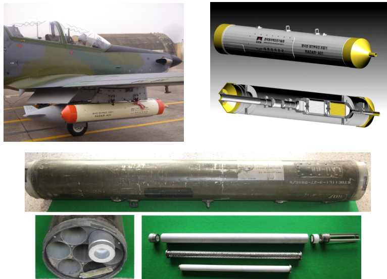
Fig. 5.4 Tactics control fighter(KA-1), the Radioactive Airborne Dust Archive for Aircraft (RADA-A) v.1 and v.2
