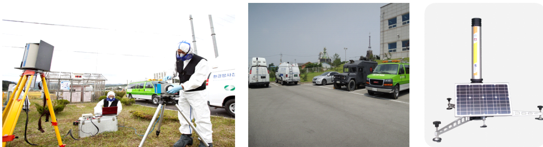
Fig. 5.10 Field radiation survey and MMP(Mobile Monitoring Post)
